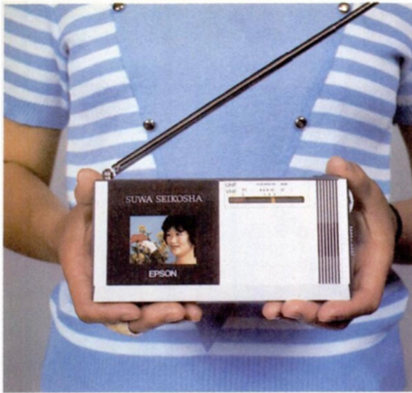
Tiny Seiko TV is slightly more than one in. thick. Measurements of the prototype are 6.3 by 3.15 by 1.1 in. It weighs 17.6 oz. Playing time is four hours on four AA alkalines.
