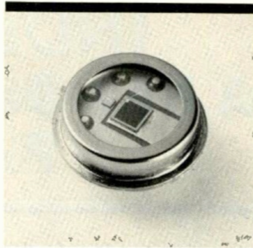
The new high-speed photodetector which makes beam indexing feasible.
