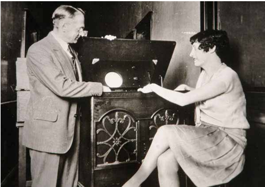
Fig. 12. Zworykin demonstrates a television receiver with a cathode-ray tube in 1928. ( http://www.earlytelevision.org/zworykin_receiver.html )
