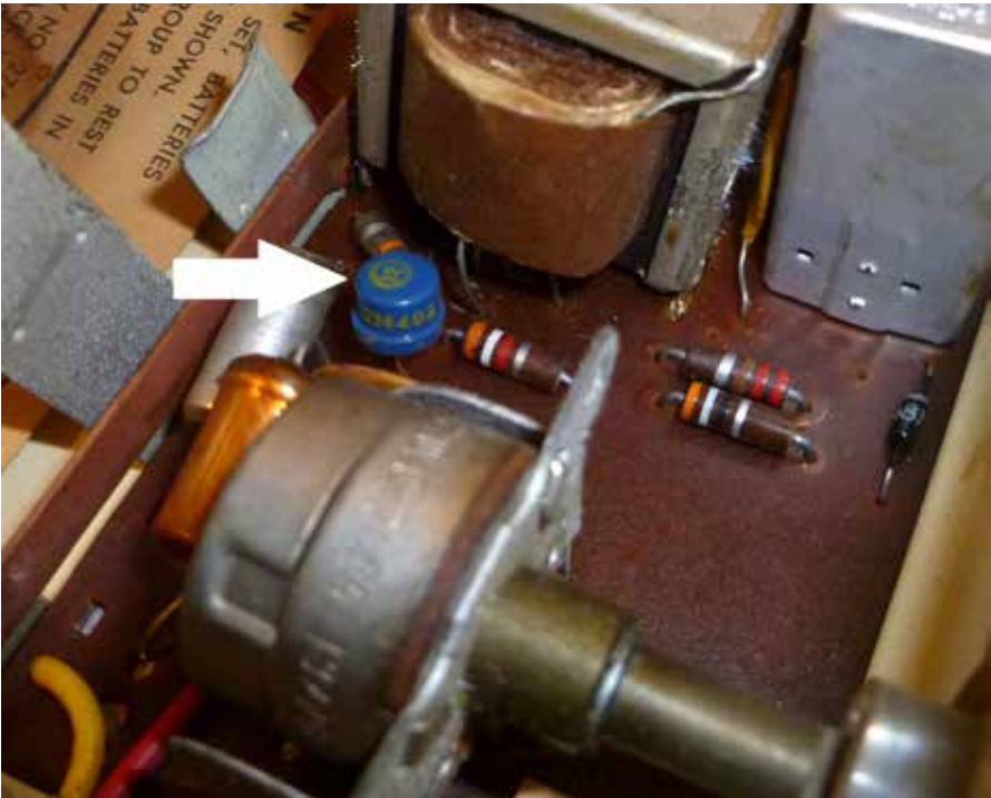
Fig. 21. Westinghouse transistor mounted on a chassis. (Author's collection)
