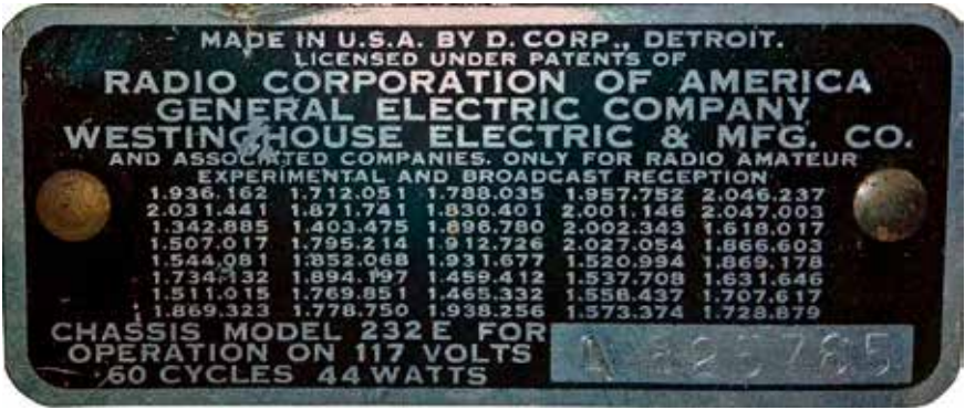
Fig. 9. A license tag found on a Westinghouse WR-262 indicates it was manufactured by Detrola Corp. of Detroit. (Courtesy of eBay advertisements)
