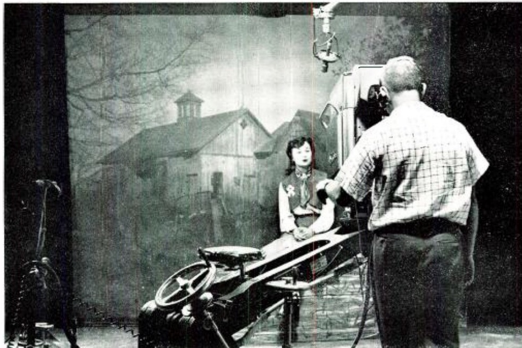
FIG. 16. Rear Projection in use on a WTMJ-TV studio program. To date it has not been used for color. However, WTMJ-TV engineers feel that they will be able to work out a method of using it, despite higher base lighting needed for color.
