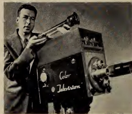
Dr. Paul K. Weimer, RCA engineer, is shown holding an experimental single tube unit for the taking camera in the RCA tri-color television broadcasting system. Called an iconoscope, or orthicon, the tube is expected to do the work of the three tubes now used. The CBS system uses a single tube for broadcasting color, separating the three colors by means of a color wheel. Circuitry for the single tube is simpler than for three guns, according to both CBS and RCA engineers.
