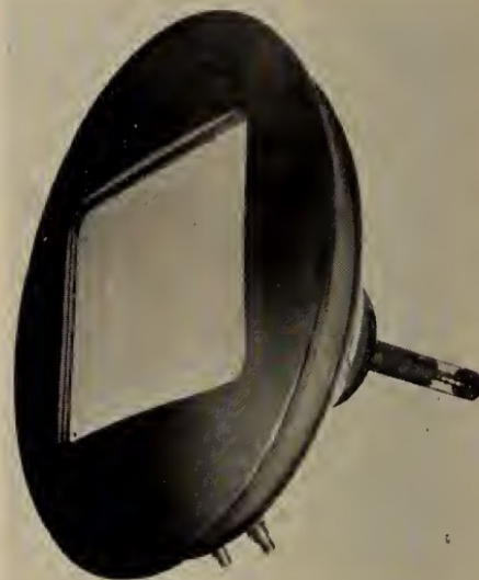
This is an early experimental Chromatron, or Lawrence tube. Production models for 21" and 24" color pictures will be rectangular at the face plate instead of round. Note the short distance between the cathode in the neck of the tube and the phosphor face plate.
